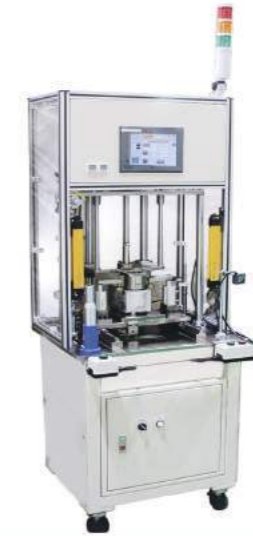
機種配對(條碼掃描) Workpiece pairing by using barcode
