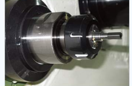
擠光刀具0.6S 0.6S Burnishing tool
