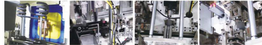
高週波機加熱鐵芯 High frequency heating lamination 矽鋼片厚度檢測 Lamination thickness detection 軸芯脫拔力測試 Shaft pull-off tester 偏擺測試機 Run-out test
