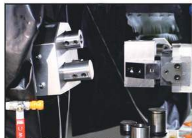
伺服控制傾斜主軸 Servo control the spindle tilt
