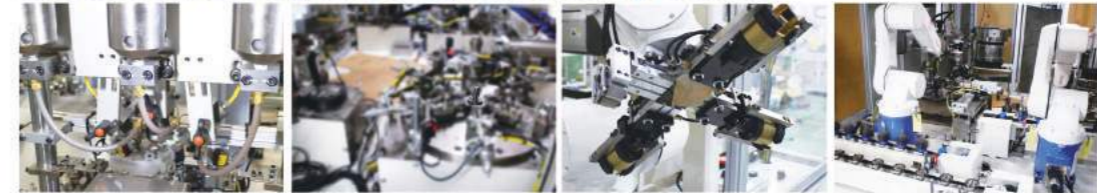
塗膠 Glue instillation 組入磁鐵 Magnet fitting 組入扣環 Circlip press fit by robot 多關節機械手協同合作 Two manipulators are cooperation
