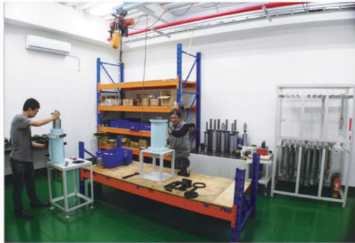
精密組裝室 Precision Assembly Workshop 配備空調設施，穩定主軸組裝精度 The shop equips with air conditioner to keep precision of spindles assembling
