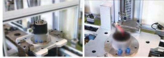
粉塵清潔 Dust cleaning the stator and the internal body 置入波形墊圈 Place in wave washer
