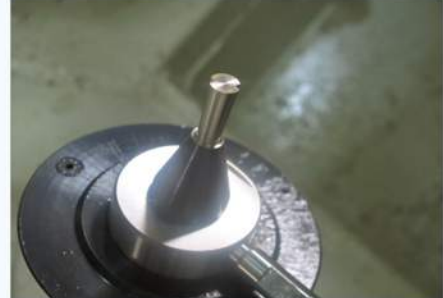
沖異型孔 Punching of asymmetrical holes
