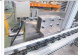
使用條碼分辨料號 Using the bar code to distinguish workpiece
