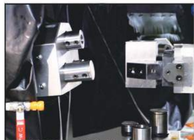
伺服控制傾斜主軸 Servo control the spindle tilt
